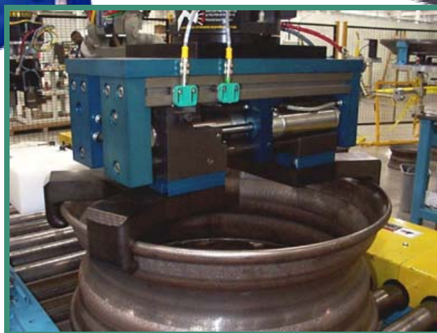
A Tandem XRAY manages a 125 lb truck wheel
